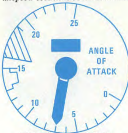
B-58 angle of attack display.
