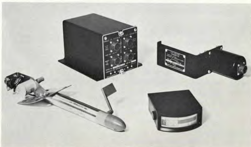
Components of angle of attack system installed in C-123 and C-130 aircraft.
